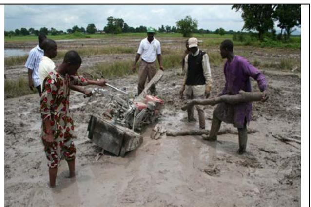
Fig. 21 (2): Power tiller stuck and overturning risk on liquefied ground. High risk even with cage-whale attachment.
