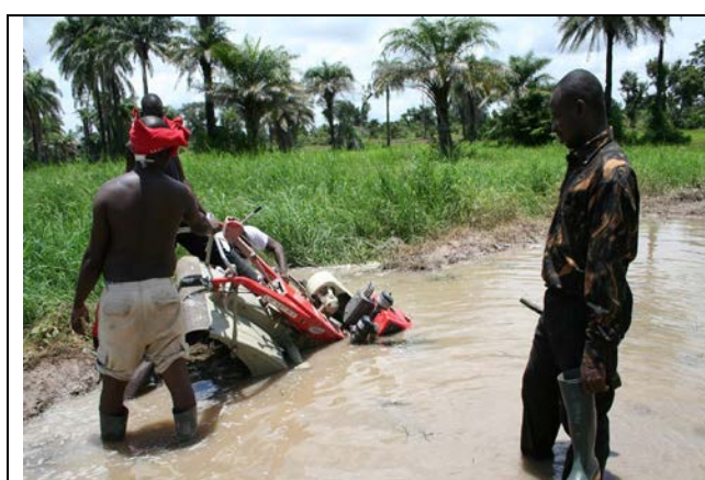
Fig. 21 (1): Power tiller stuck and overturning in hole under muddy water. Is risk avoidable with sturdy cage-whale attachment?
