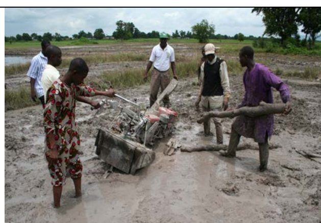
Fig. 21 (2): Power tiller stuck and overturning risk on liquefied ground. High risk even with cage-whale attachment.
