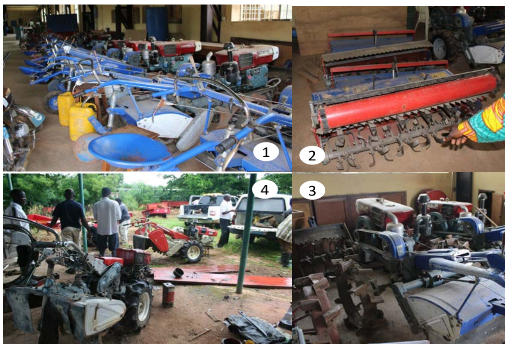
Fig. 6. Powertillers supplied by JSPS fund (Wakatsuki 2007-12, and 2013- and 2018) for Sawah Technology training at Kebbi, Ebonyi, FCT, Benue, Delta and Lagos states during 2010-2015. ① 12 sets of Dong Feng powertiller ready to deploy to the six states at NCAM storage warehouse. ② Rotavators are suitable for puddling that have already been developed. As shown in Fig.21④, ploughs are more efficient for new sawah development. ③ Anti-skid wheels are suitable for upland and lowland areas with relatively firm ground. As shown in Figures 9③ and 21④, Cage-wheel is more suitable for wetlands with soft muddy soils. ④ Other power tillers used for other Sawah project Shakti from India and Kubota/Japan, at NCRI storage.
