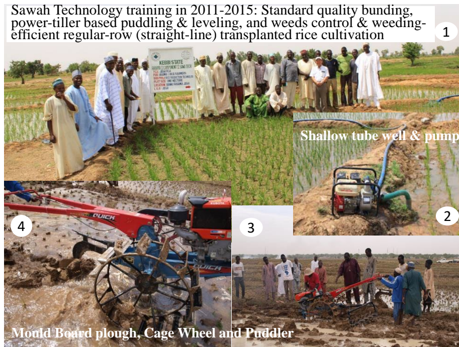
Fig. 22. Some scenes of Sawah technology training and demonstration at Kebbi. ① and ② are demonstration plots at Jega site 1, May 2011. ③ and ④ are advanced sawah technology training using KHS Indonesia's Quick G1000Bower power tillers (11 Hp equipped with Kubota engine) attached a mould board plough, puddler, leveler and cage wheel, at AR2 site, Arugungu, in July 2015.
