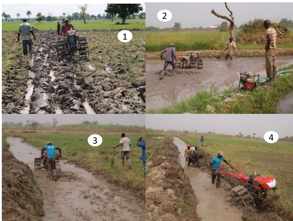
Fig. 24 ① and ④: A plow and wetland cage wheels can be attached to power tiller to work in conjunction with the farmer's hoeing operation to streamline the work of creating larger bunds for flood control and cutting waterways. Farmer can use it in place of a backhoe. Fig.24②: A leveler and plow are attached to the power tiller to fluidize (so called thixotropy) and level the soil and efficiently cut drainage channels as shown in ③. The soil can be moved 10-30 m, replacing a bulldozer. Photo taken near Gbajigi village, Edozhigi irrigation scheme, Bida, Niger state, 2015-2017.
