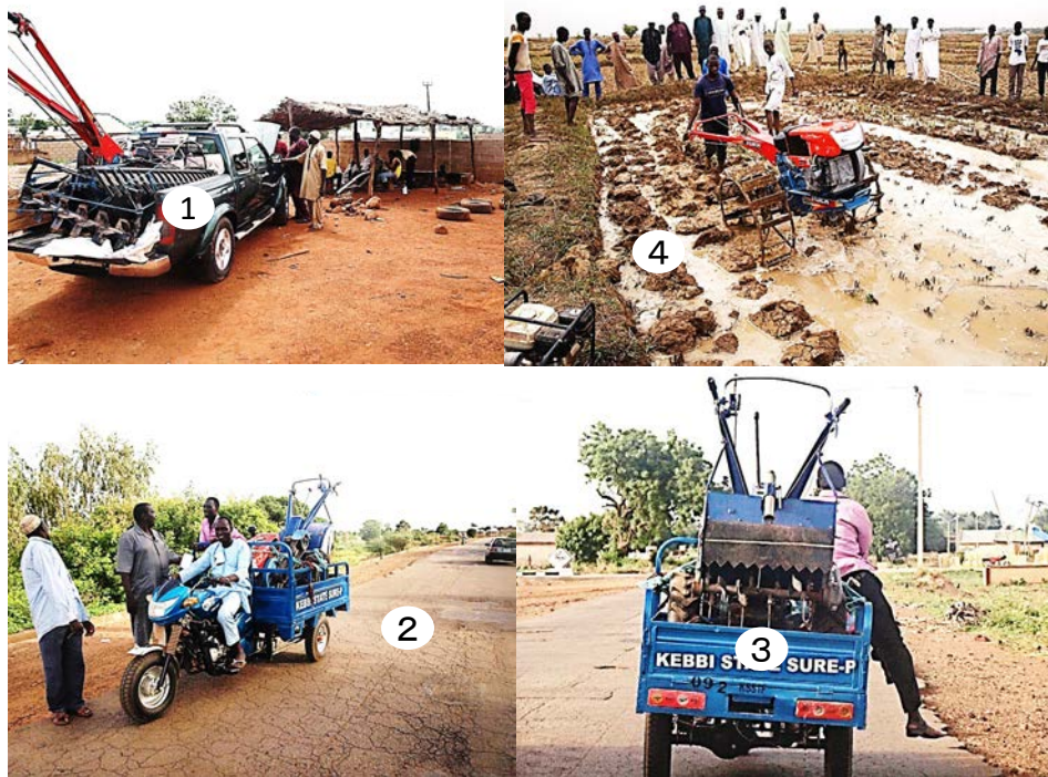
Fig. 28: Sawah Technology's upgraded technical training on July 8-12, 2015. ①: KHS G1000boxer power tiller to Kebbi state on a pickup truck along with puddler, leveler, and cage wheels. ② and ③: A heavy Chinese-made Dong Feng (570 kg, 15 HP) power tiller can be transported to any small village in Kebbi state by towing a cart on a motorcycle. ④: Mould board ploughing operation by KHS G1000boxer power tiller.
