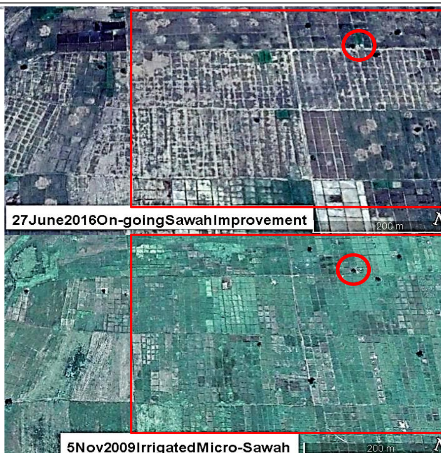
Fig 12b. Evolution of Maigandu Sawah system (Fig 6&7 shows the position) is on-going after Sawah technology training in 2011-2015 using power tiller by NCAM sawah team (both are Google earth). Each Two red tetragram area has 12ha, in which about 2200 micro sawah plots exist, mean area is 55m 2 in 2009, while total sawah plots reduced to about 450, mean area expand to 270m 2 in 2016. Red circles show the position of photographs in Fig 11. Expansion of sawah plots resulted through improvement of bunds' quality for both water control and operations. Leveling quality of sawah soil surface was improved. These sawah evolutions improved intermittent irrigation efficiency and gave paddy yield, double 2-3 to 5-7t/ha.
