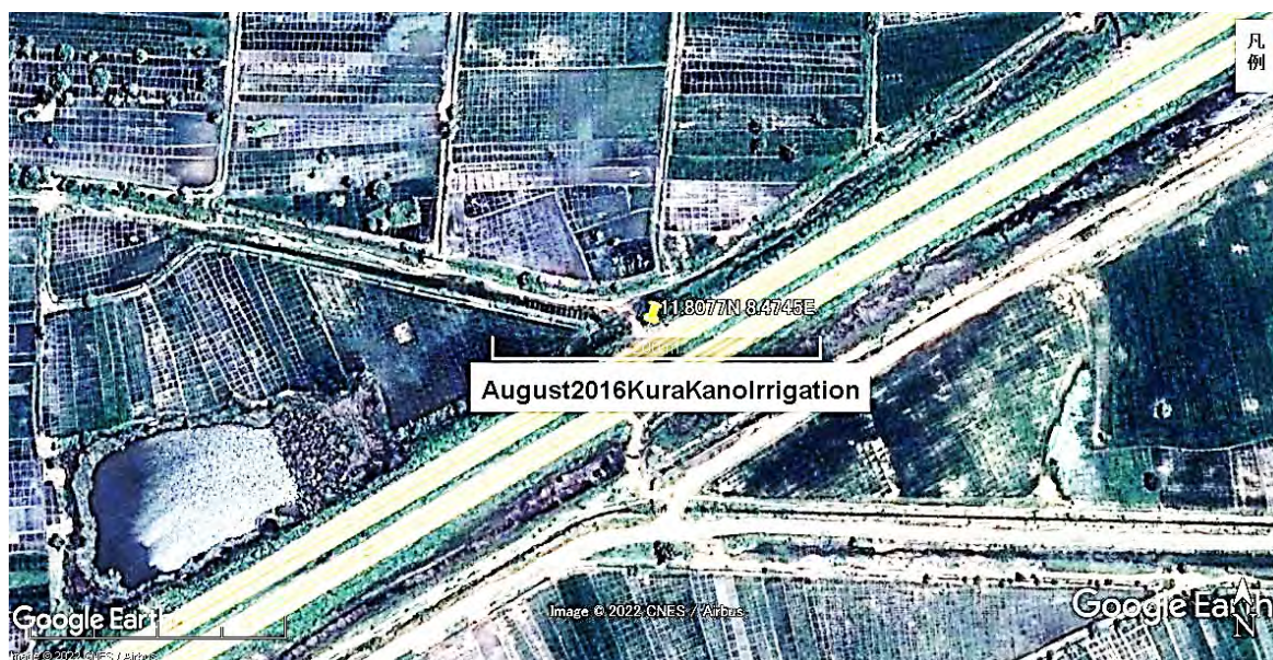
Figure 9. Google earth image of Kura site of Kano Irrigation Scheme at the 11.8077N 8.4745E position on 20, August 2016, showing that all the irrigated platforms are micro-rudimentary Sawah plots of size 20–30 m 2 (The central marker is 200m long)
