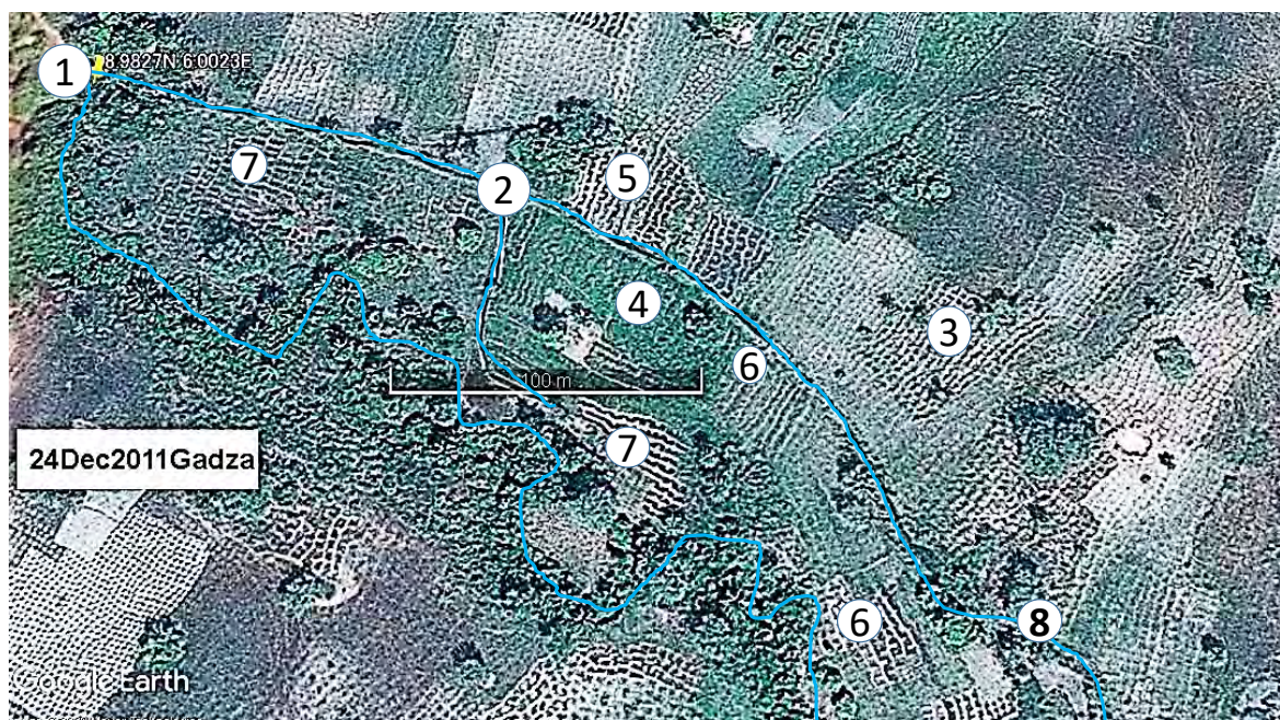
Figure 2. Expansion of the yellow square area of Figure 1. Various irrigated and rainfed rice platforms, that is., ① Irrigation weir by Bida Agric Development project managed by Gadza farmers, ② Irrigation canal ③ Spring and ④ Weir irrigated micro-rudimentary Sawah system, ⑤ Spring and ⑥ Dyke irrigated ridge/micro-Sawah, and ⑦ irrigated ridge rice planting
