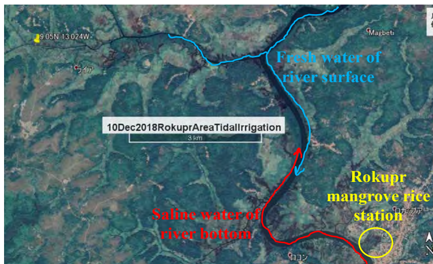
Figure 4: Tidal Irrigation system of the coastal wetlands and river system along the Gulf of Guinea. The upper left yellow pin shows GPS position (9.05N 13.024W) and the lower right yellow circle shows Rokupr Mangrove Rice Research station of WARDA, Sierra Leone.
