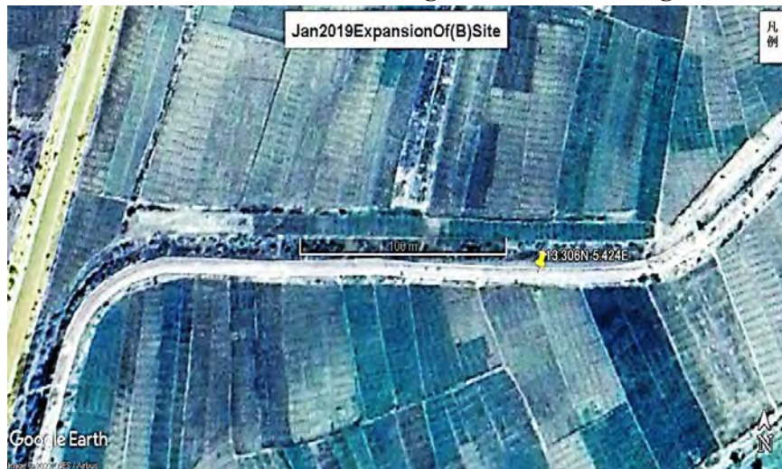
Figures 11B: Expansion of the location (B): 13.306N 5.424E, showing ridge rice cultivation platform of official irrigation schemes. The white curve from north east to south west in the center has the farm road, irrigation/drainage canal. The straight line shows major road.
