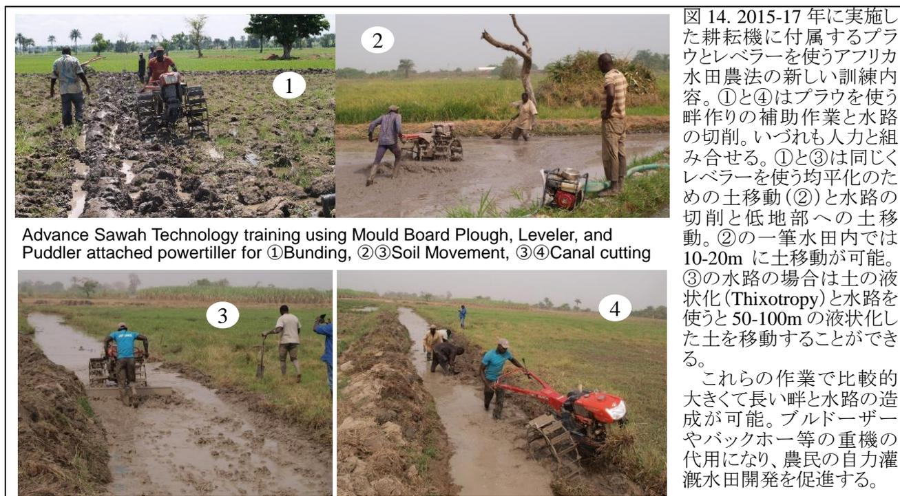
Advance Sawah Technology training using Mould Board Plough, Leveler, and Puddler attached powertiller for ①Bunding, ②③Soil Movement, ③④Canal cutting
