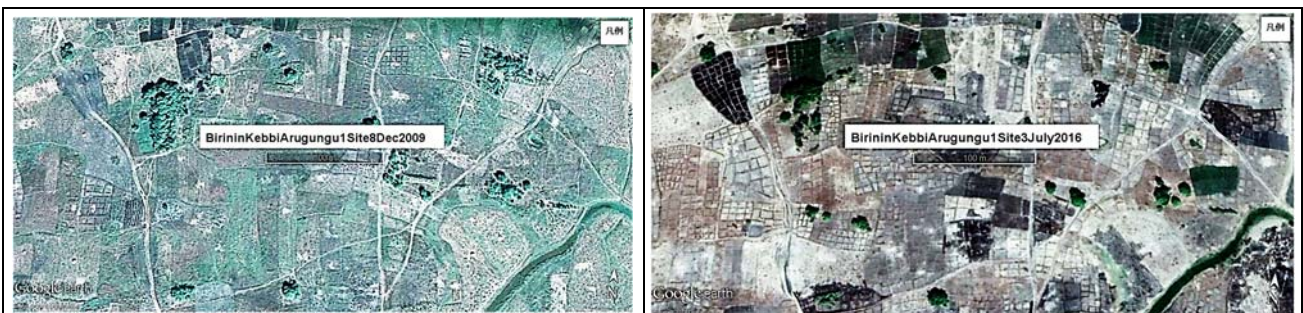
Figure 26. Evaluation of the progress of sawah platform improvement on 2009 (left) and 2016 (right) by Google images near Site 1 of the Rima River floodplain shown in Figure 22. The total area shown is 10 ha. The length of the scale marker is 100 m. In 2009, 10% area is rudimentary sawah field and remaining is non sawah fields. In 2016 sawah platform improvement began and standard sawah plots covered about 80% of the flood plain. Mean sawah plots size in 2016 is about 60\text{ m}^2
