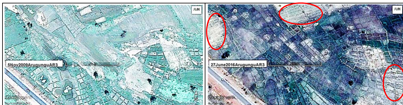
Figure 20. Progress of sawah platform during 2009 (left) and 2016 (right) by Google earth at Arugungu (AR3) site (Fig. 13). Scale marker is 100 m and area is 10ha. In 2009, 10% land is rudimentary sawah plots and remaining is non sawah fields. In 2016, 80% land are improved standard sawah plots with good bunding and leveling. 10% land, which are shown in three red circles, are ridge rice planting. Mean sawah plots size in 2016 is about 120 m 2 .
