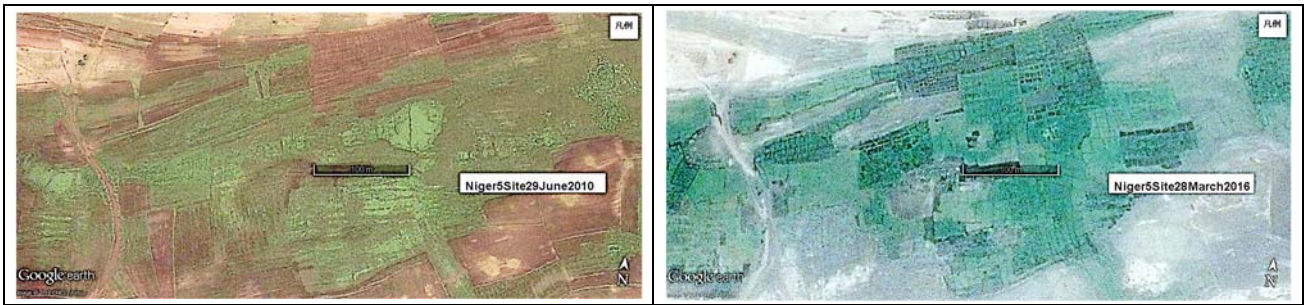
Figure 87. Progress of sawah platform improvement between 2010 (left) and 2016 (right) which appeared in Google earth image near Site 5 in Figure 80. The site is a part of Niger rive flood plain. Total area shown is about 10 ha. Scale marker length is 100 m. In 2010, 100% area has no sawah system. In 2016, although still rudimentary, sawah system is expanding to 50 % area (mean sawah plot size is 40m 2 ).
