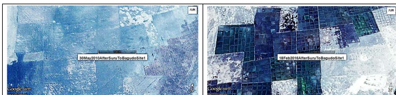
Figure 65. Progress of sawah platform improvement between 2010 (left) and 2016 (right) which appeared in Google image near Site 1, which is just south of Suru town, downstream of the Rima River floodplain shown in Figure 64. The total area shown is about 10 ha. The length of the scale marker is 100 m. In 2010, 100% flood plain has no sawah
