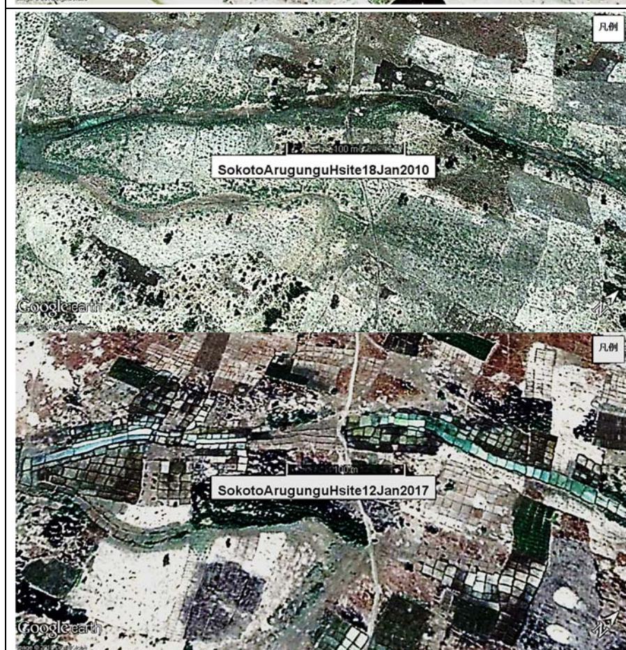
Figure 5. Evaluation of the progress of sawah platform improvement in 2010 (above) and 2017 (below) by Google earth images at the floodplain H (Fig.2) near the Sokoto state boundary. The total area shown in the photograph is about 10 ha. The length of the scale marker is 100 m. In 2010, almost no sawah plots are recognized. In 2017 about 80% of this flood plain are occupied by sawah plots, mean size about 100 m 2 . These were developed by farmers' self-help efforts, which is clear all sawah plots are developed based on the land use demarcation of 1 acre to 1ha size. It is impressive that almost all seasonal river bottoms are occupied by sawah plots.
