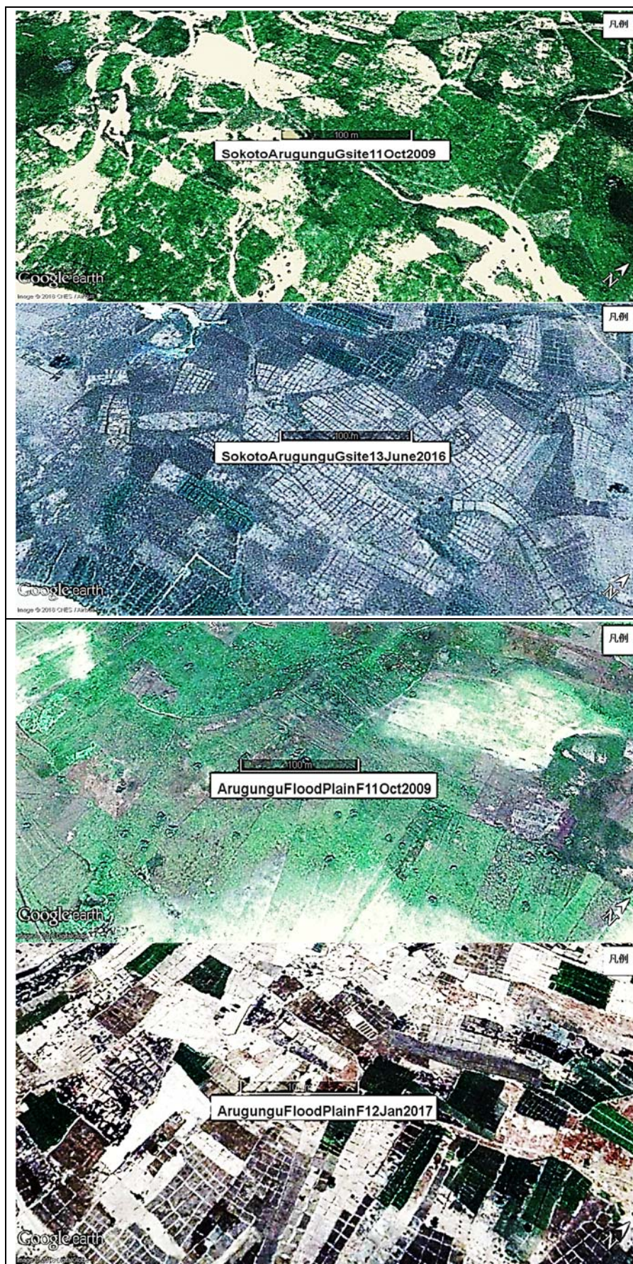
Figure 6. Evaluation of the progress of sawah platform improvement in 2009 (above) and 2016 (below) by Google earth images at the floodplain G (Fig.2). This location is the area approaching to the rice center of Kebbi, i.e., Arugungu. The total area shown in the photograph is about 10 ha. The length of the scale marker is 100 m. Almost 100% of the flood plains were occupied by ridge rice cultivation in 2009. In 2016, however, sawah plots based rice farming became major although still micro sawah plots and less than 50 m 2 size and ridge rice cultivation. The sawah bunds are strengthened and clearly identified.
