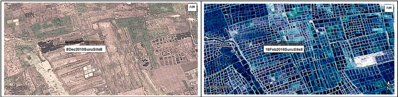
Figure 59. Progress of sawah platform improvement between 2010 (left) and 2016 (right) which appeared in Google image near Site 8 in Suru area of of the Rima River floodplain shown in Figure 50. The area is about 10 ha. The scale marker is 100 m. In 2009, 90 % land have no sawah system and 10% rudimentary sawah system. In 2016, 100% land is covered with sawah system (mean sawah plot size is 100m 2 ).
