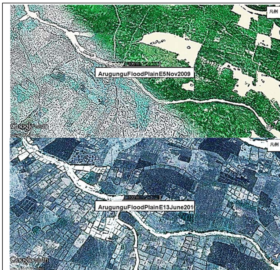
Figure 8. Evaluation of the progress of sawah platform improvement in 2009 (above) and 2016 (below) by Google earth images at the floodplain F (Fig.2) near Arugungu floodplain E. The total area shown in the photograph is about 10 ha. The length of the scale marker is 100 m. In 2009, non-sawah rice fields and ridge rice cultivation were all over the flood plain. In 2016, 70% area are covered with standard sawah plots of 100 m 2 mean size. The rest areas are non-sawah and micro rudimentary sawah.
