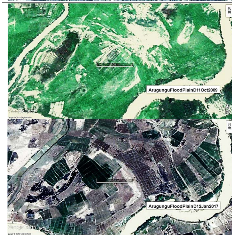
Figure 9. Evaluation of the progress of sawah platform improvement in 2009 (above) and 2016 (below) by Google earth images at the floodplain F (Fig.2) near Arugungu floodplain D. The total area shown is about 10 ha. The length of the scale marker is 100 m. In 2009, although more than 80% are non sawah, it can be seen that the development of micro rudimentary sawah system started with 5 places of floodplain, each 0.5-1 ha. In 2016, more than 80% area are covered with sawah plots, mean size is about 70 m 2 , with clear bunding systems. But still some minor areas have ridge rice planting.
