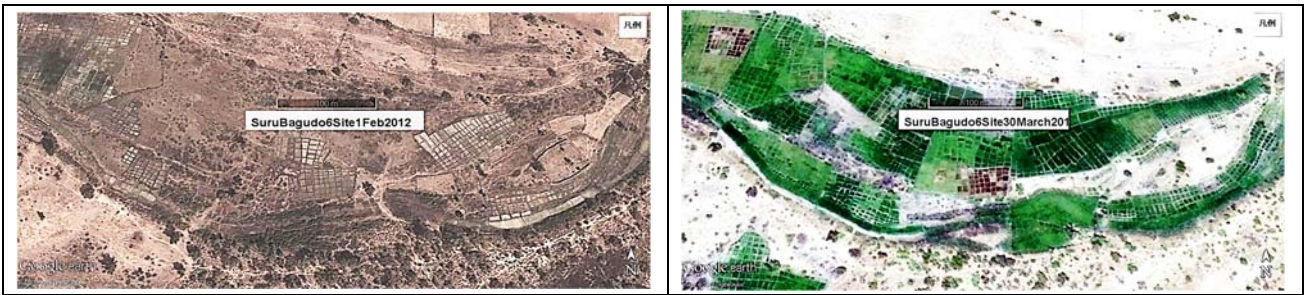
Figure 70. Progress of sawah platform improvement between 2012 (left) and 2014 (right) which appeared in Google image near Site 6 of the Rima River floodplain shown in Figure 64. The total area shown is about 10 ha. The length of the scale marker is 100 m. In 2012, 20% flood plain has covered with micro rudimentary sawah system (mean sawah plot size is 30m 2 ). In 2016, 40% land is covered with sawah system (sawah plot size range is 20-70m 2 ).
