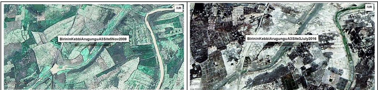
Figure 25. Evaluation of the progress of sawah platform improvement on 2009 (left) and 2016 (right) by Google images near A3 site of the Rima River floodplain shown in Figure 22. The total area shown is 10 ha. The length of the scale marker is 100 m. In 2009, all area is non sawah field. In 2016 sawah platform improvement began and standard sawah plots covered about 70% of the flood plain. Mean sawah plots size in 2016 is about 100\text{ m}^2
