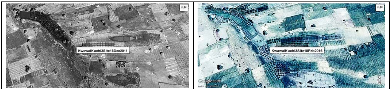
Figure 74. Progress of sawah platform improvement between 2011 (left) and 2016 (right) which appeared in Google image near Site 3 of the Ka River floodplain shown in Figure 70. The total area shown is about 10 ha. The length of the scale marker is 100 m. In December 2011, sawah system development is proceeding in 10% area, the others are ridge rice cultivation and non-sawah, in 2016 although still rudimentary level, sawah system is expanding to 20-30 % area (mean plot size is 50\text{m}^2 ). Remaining 80-70 % is ridge rice cultivation.
