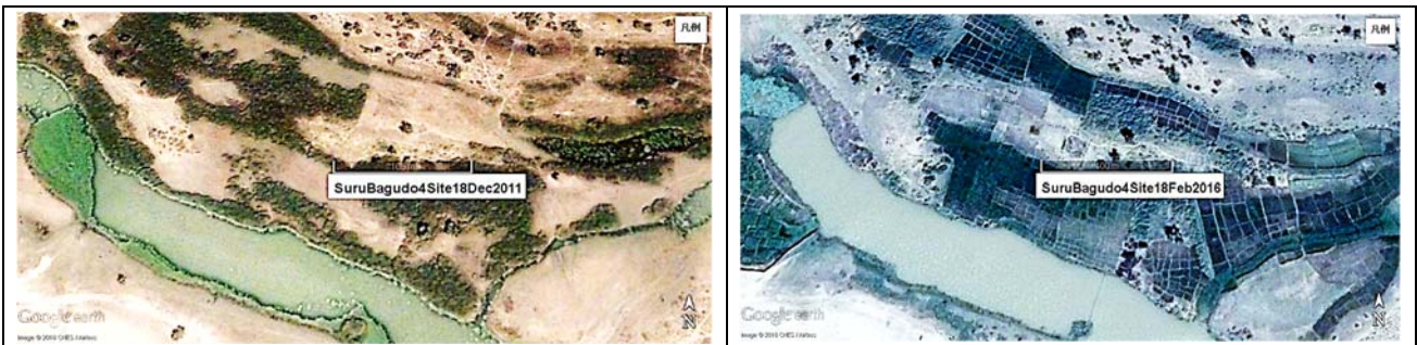
Figure 68. Progress of sawah platform improvement between 2011 (left) and 2016 (right) which appeared in Google image near Site 4 of the Rima River floodplain shown in Figure 64. The total area shown is about 10 ha. The length of the scale marker is 100 m. In 2011, 100% flood plain has no sawah system. In 2016, 30% land is covered with sawah system (mean sawah plot size is 80m 2 ).
