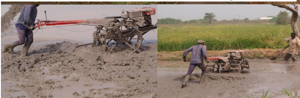
Indonesian G1000 Boxer can move soil 25m for leveling(10 th Dec 2015)
