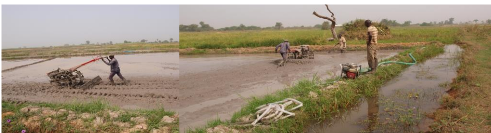
Indonesian G1000 Boxer can move soil 25m for leveling(10 th Dec 2015)
