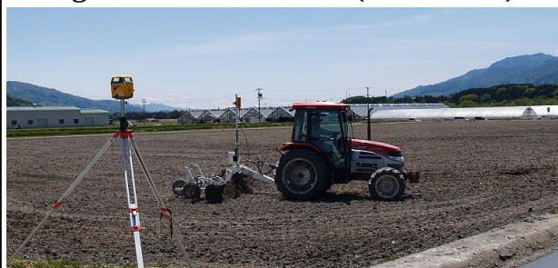
6 th Stage: Advanced and large sawah plot of >1\text{ha} with leveling quality of \pm 2.5\text{cm} using laser leveler tractor (Kubota Co)
