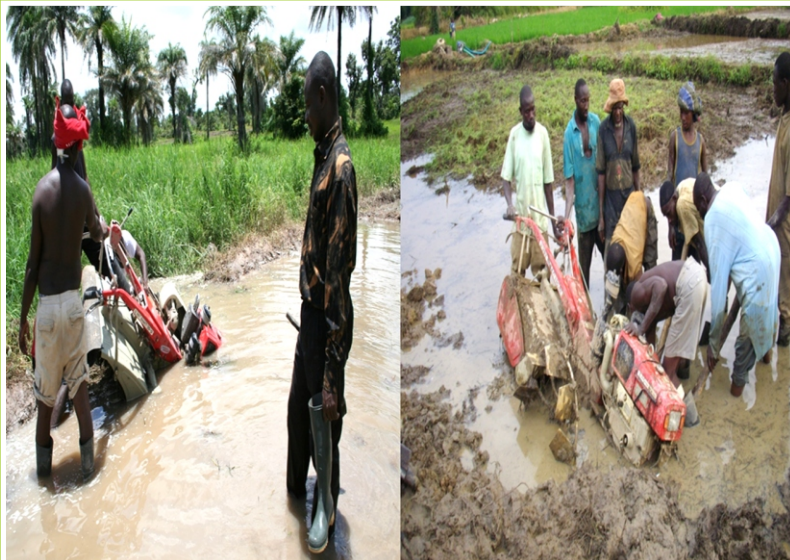
Common field problems when using the power tiller include sinking into too soft lands or old sunk wells. As much as possible such situations should be avoided as they tend to damage machinery
