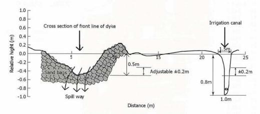
Fig. 18. Ajustable canal flow system using sand bags.
