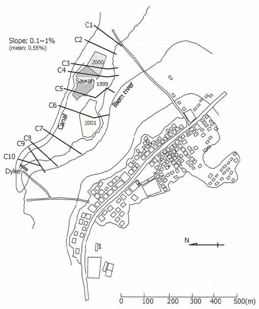
Fig. 15. Biemso No.1 sawah system with cross section lines (C1~10).
