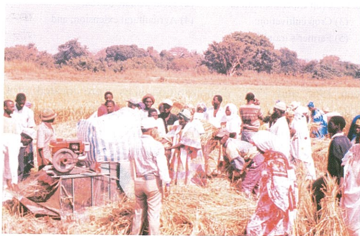
Fig. 9-12. Inexpensive rice thresher from Taiwan was introduced to Domasi rice plantation in Malawi. The small motor operated semi-automatic rice thresher is not only cheap in price, but also very efficient in grain threshing.
