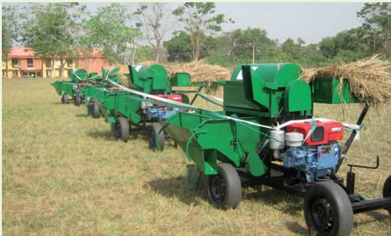
The ATAT thresher–cleaner produced by trainees at NCAM, Ilorin
