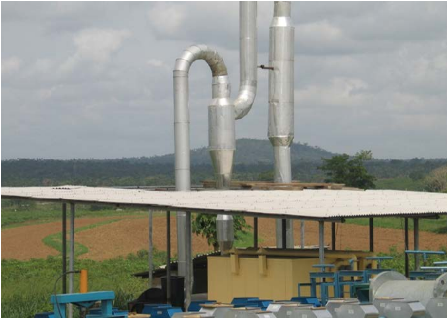
Figure 32: Flash dryer of a small (one metric tons per day) HQCF mill. Upgrades of these mills to large and more efficient flash dryers is a major component of the cassava transformation
