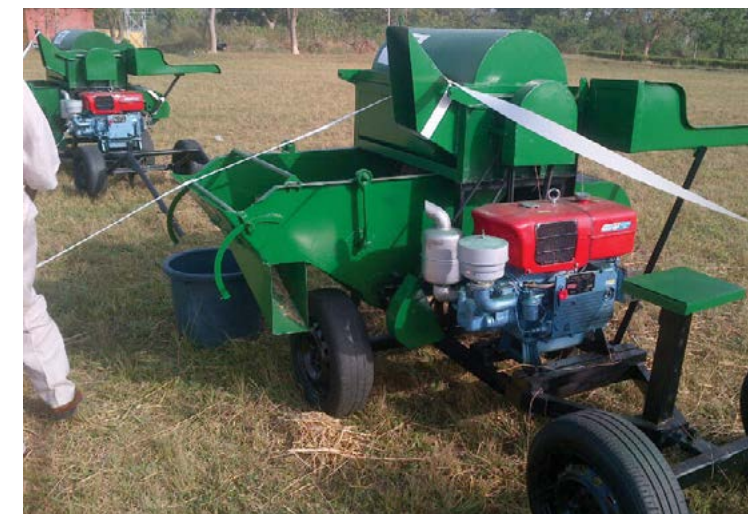
Figure 22: The new rice thresher fabricated during a training workshop of Africa Rice Center in Ilorin
