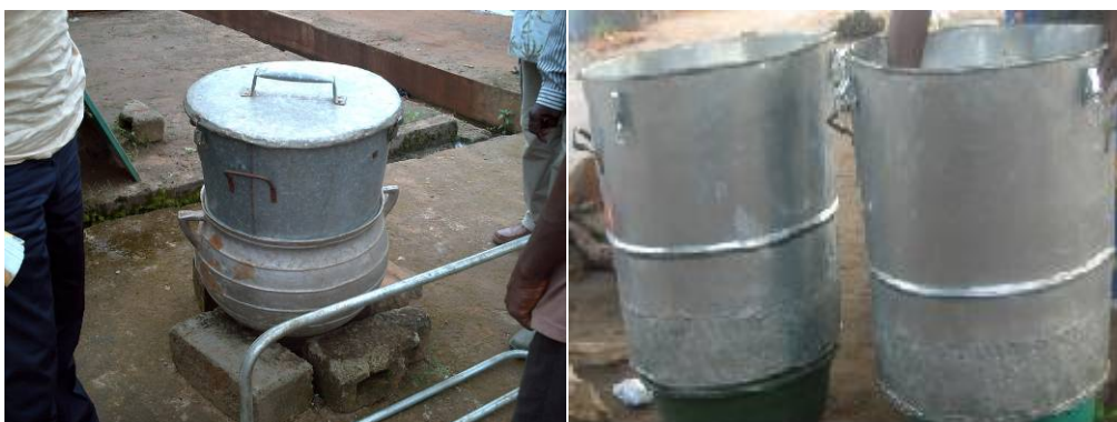
Figure 1. Improved parboiling equipment used for the study: (A) general shape of the improved parboiler; (B) the steaming vat.
