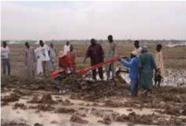
Indonesian G1000 Boxwer's puddler, leveler and plow. Plow can help bunding (10 th Jul 2015), Kebbi and Niger State, Nigeria
