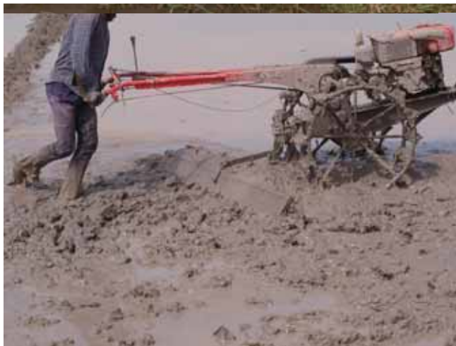
Indonesian G1000 Boxer can move soil 25m for leveling(10 th Dec 2015)
