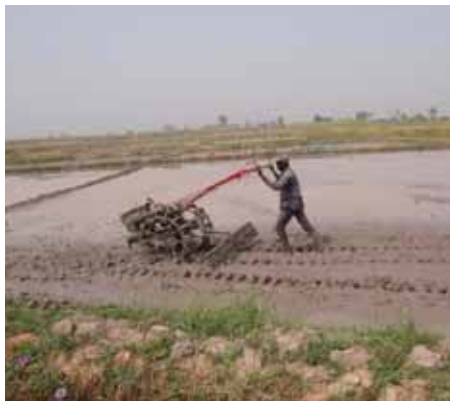
Indonesian G1000 Boxer can move soil 25m for leveling(10 th Dec 2015)
