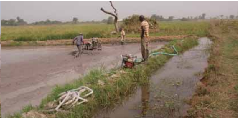
Indonesian G1000 Boxer can move soil 25m for leveling(10 th Dec 2015)
