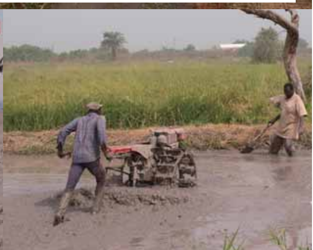
Indonesian G1000 Boxer can move soil 25m for leveling(10 th Dec 2015)
