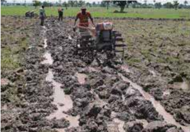
Indonesian G1000 Boxwer's puddler, leveler and plow. Plow can help bunding (10 th Jul 2015), Kebbi and Niger State, Nigeria
