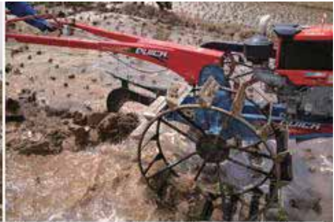
Indonesian G1000 Boxwer's puddler, leveler and plow. Plow can help bunding (10 th Jul 2015), Kebbi and Niger State, Nigeria
